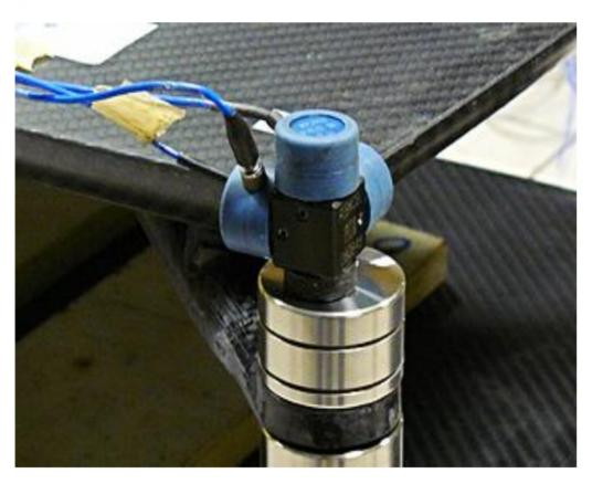
We have used a measuring hammer and four mono-axial accelerometers on 51 selected points so to recreate the structural net.
