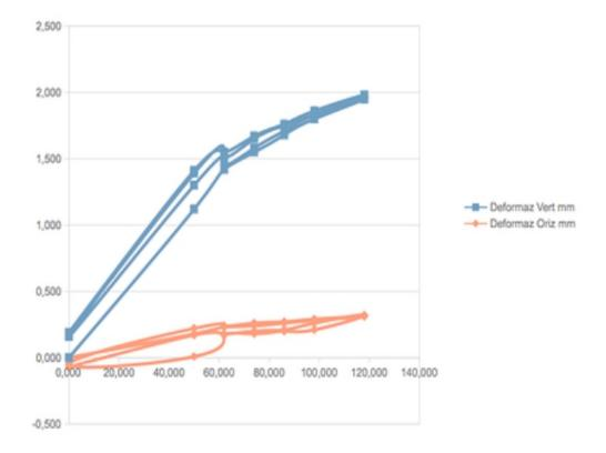
The deformation curves show a straight trend and a very high static resistance. The deformation is inferior to 2 mm on a 800mm long arm, loaded in its central part with more than 120 kg. With the same load the horizontal deformation is inferior to 0,3 mm.
