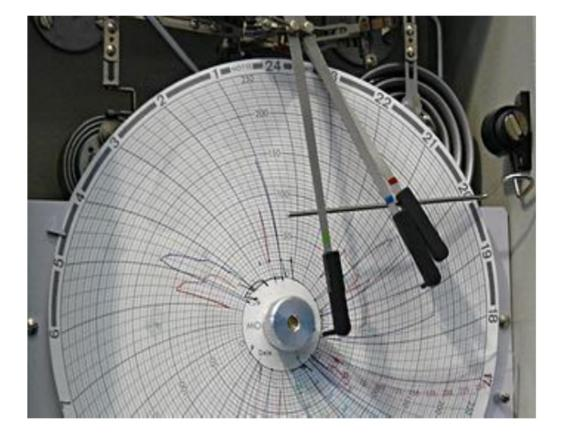
High temperature and pressure (120 C° and about 6 bars) inside the mould facilitate the hardening of the epossidic resin and the absence of air bubbles in the structure.
